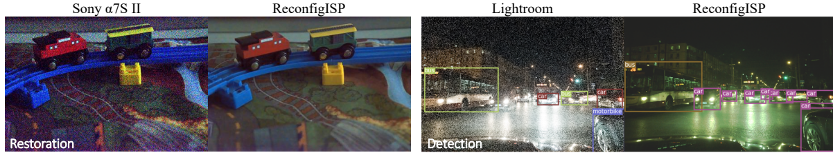
Figure 1: While inheriting the modularity of traditional ISP, ReconfigISP can adapt to different tasks, such as image restoration and object detection by learning to reconnect specialized ISP modules. For each task, the left image shows the results of a default camera processing pipeline while the right image presents our output (zoom in for best view). In the task of object detection, ReconfigISP optimizes the ISP for more accurate detections rather than perceptual quality.
