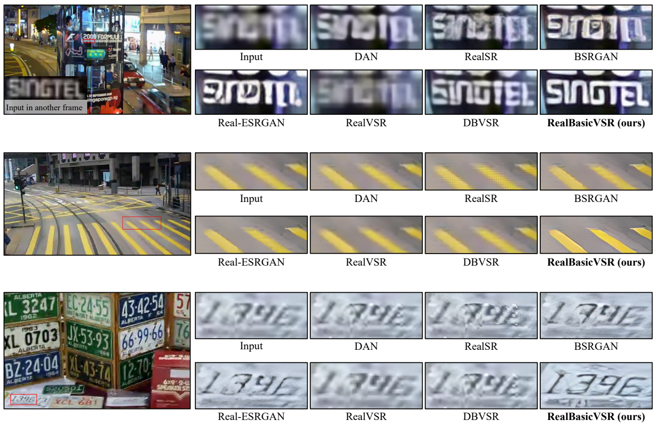
Figure 2. Qualitative Comparison. By employing the long-term information effectively, RealBasicVSR restores more details when compared to existing state of the arts. ( Zoom-in for best view )
